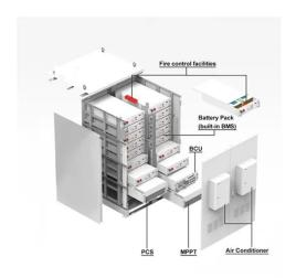
is composed of battery cabinet and electrical cabinet. It can apply to demand regulation and peak shifting and
